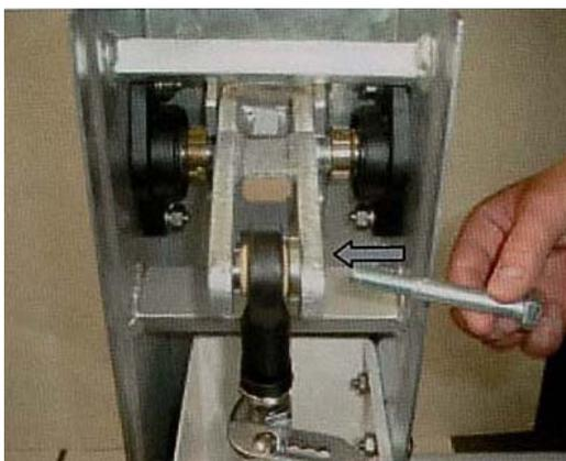
6) Place screw into lever socket and linkhead with bolt
