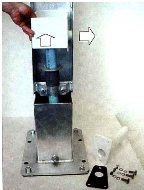
1) Position the water tank into pump body
