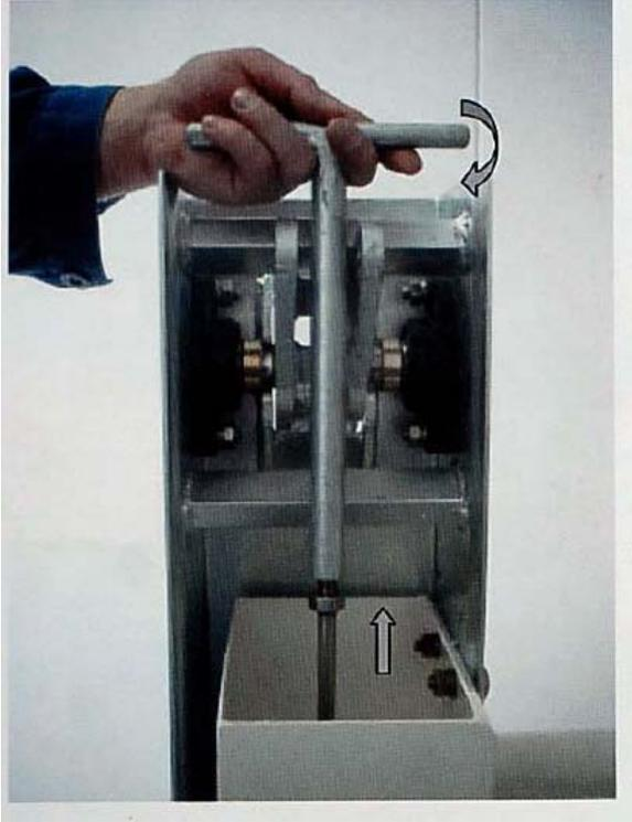
1) Screw T-bar onto the rod.
