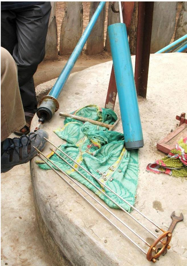
1) Once all cylinder components have been checked and cleaned, reassemble them
