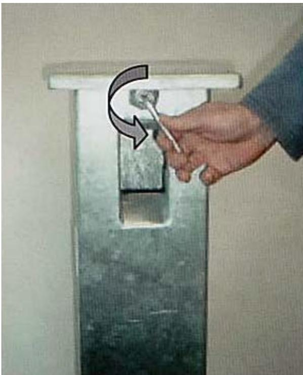
1) Unscrew Allen screw from pump body
