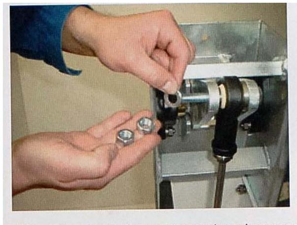
7) Take pliers off and place washer and one hexagonal nut on bolt
