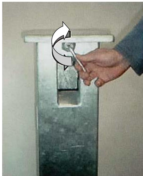
2) Screw Allen screw on the pump body
